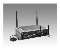
The NVR features up to  $4 \times 10/100$  Mbps -4 ports full-load, IEEE802.3af Class 2 (7 Watt) and 2 ports full-load, IEEE802.3af Class 3 (15.4Watt). It features extended temperature peripherals of up to -40 to 70° C with relative humidity of 95 percent at  $40^{\circ}$ C, making it ideal for in-vehicle applications.
